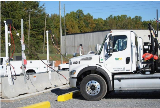
The new Waste Management CNG vehicle fueling using time-fill
